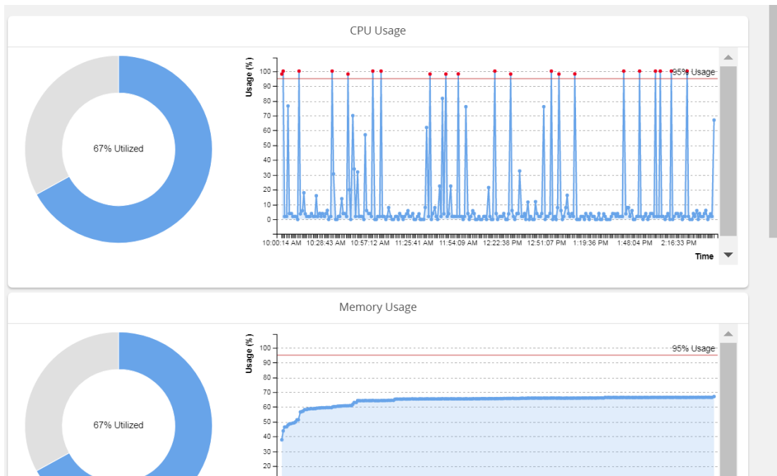
Figure 53: Health Monitor Dashboards
